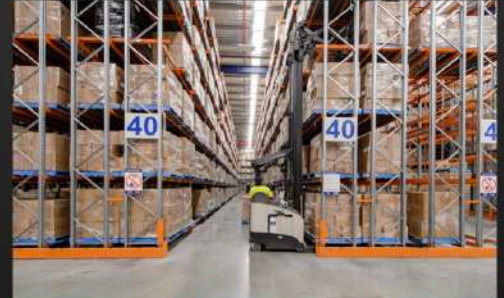
Double Deep Pallet Racks
